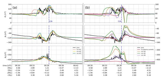
Figure 2. Magnetic field  $\underline{B} = (B_X, B_Y, B_Z)$  near Europa in EPhiO coordinates: model results versus Juno data. The figure displays time series of the observed magnetic field components (black) as well as output from AIKEF runs (a) #1–#3 and (b) #4–#6. Plot (b) also shows the magnetic field obtained from a mere superposition of  $\underline{B}_0$  and Europa's induced dipole (red). The dash-dotted blue line (labeled C/A) denotes the position of Juno's closest approach.
