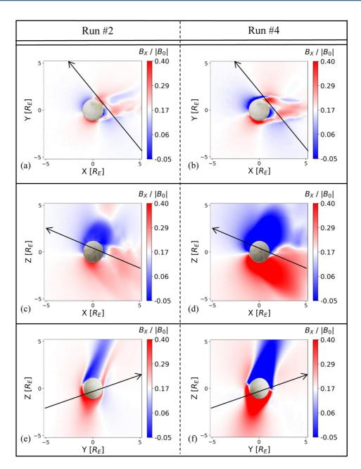
**Figure 3.** Modeled  $B_X$  components in the Z = 0 (panels (a) and (b)), Y = 0 (panels (c) and (d)), and X = 0 planes (panels (e) and (f)). Results from setup #2 are displayed in the left column, whereas the right column shows output from run #4. In all panels, white coloring corresponds to the  $B_{0,X}$  component of the magnetospheric background field. The projection of Juno's trajectory onto each cutting plane is indicated by the black line.
